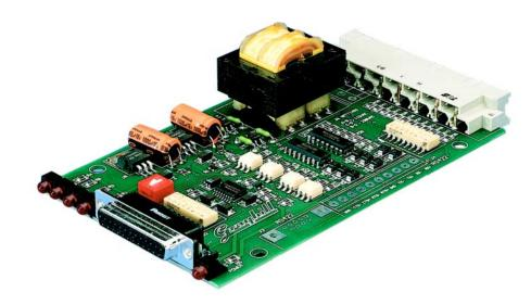
handshaking can be controlled from either end of the communication link. Typical applications involve connecting a host computer to remotely located serial devices such as printers, control equipment, or data acquisition devices distributed throughout an office or factory.
