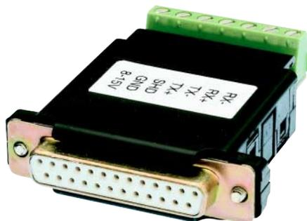
72-CNV-4 and 72-CNV-5 convert serial communications from RS-232 to RS-485 in both directions. The converter simply plugs into any male RS-232 DB-25 connector and converts the transmit and receive signals to RS-485 (RS-422) levels at speeds to 115.2 KB. The converters are configured for DTE (default) or DCE operation.
